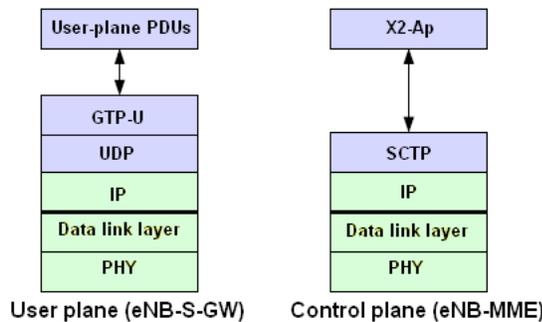
Fig. 5. X2 Interface user and control planes
