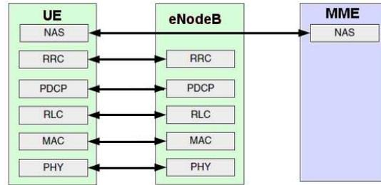
Fig. 3. Control plane protocol architecture
