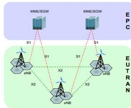
Fig.1. LTE-Advanced architecture
