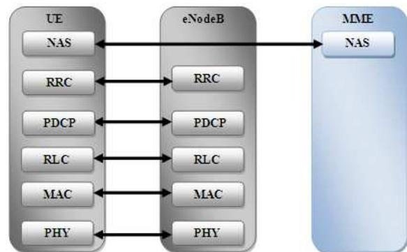
Fig. 3. Control plane protocol architecture
