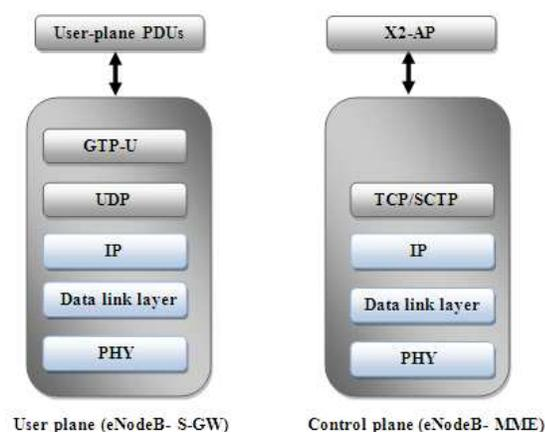
Fig.5. X2 Interface user and control planes
