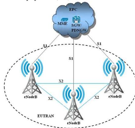
Fig. 1. LTE-Advanced architecture
