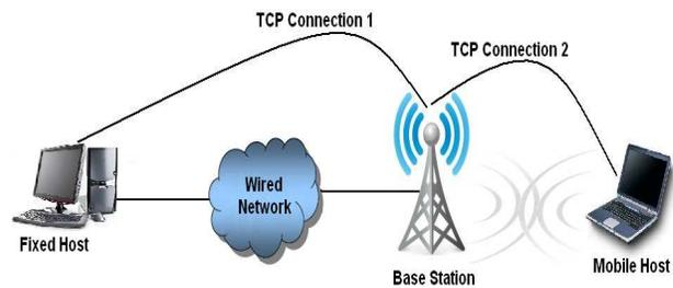
Fig.1 Splitting TCP connections into two parts
