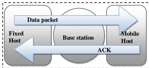
Fig. 3 End-to-end connection of a wireless TCP
