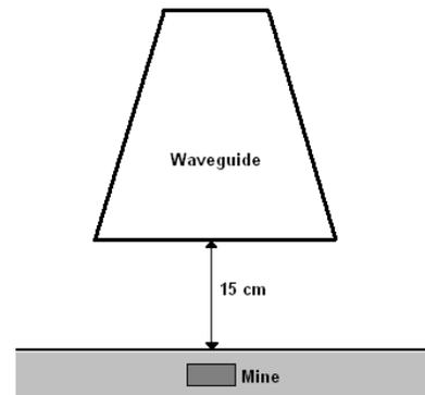
Fig. 2 Distance R from waveguide to the soil
