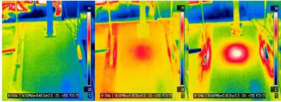
Fig. 6 Microwave heating source with buried mine buried in depth of 1 cm and after 0, 3, and 13 minutes
