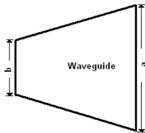
Fig. 3 WR340 waveguide dimensions
