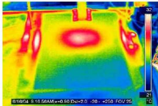
Fig. 8. Microwave heating without mine and after 15 minutes
