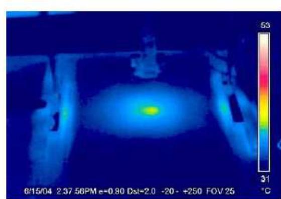
Fig. 7. Microwave heating mine buried in depth of 1 cm and 23 minutes
