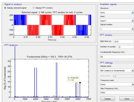
Fig. 8 Fourier analysis of the output inverter
