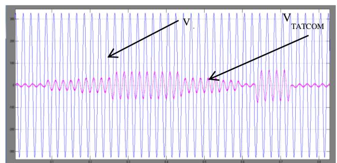
Fig. 12 The injected compensated voltage V<sub>STATCOM</sub> versus phase voltage
