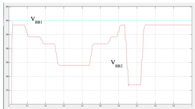
Fig. 10 The BB2 voltage without compensation
