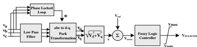
Fig. 4 Block diagram for STATCOM control system
