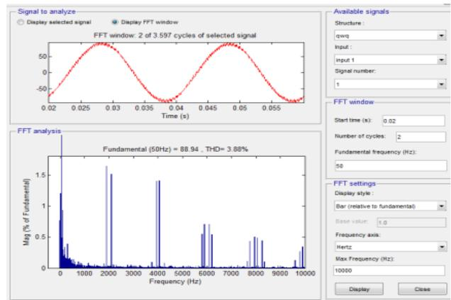
Fig. 9 Fourier analysis of the line current after STATCOM voltage injected
