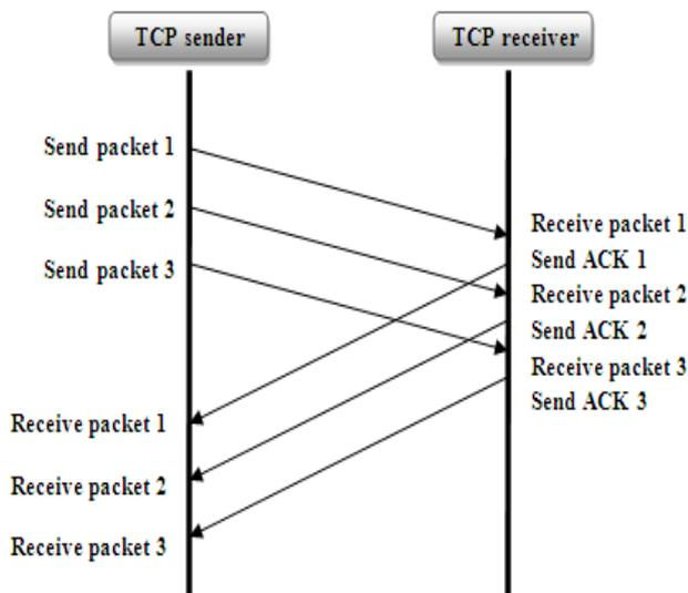
Fig. 1 Three Packets Transmitting and Acknowledging using TCP
