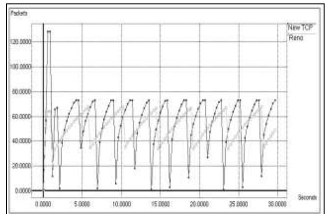
Fig.2 Behavior of new mechanism with Reno (BW=100Mbps)
